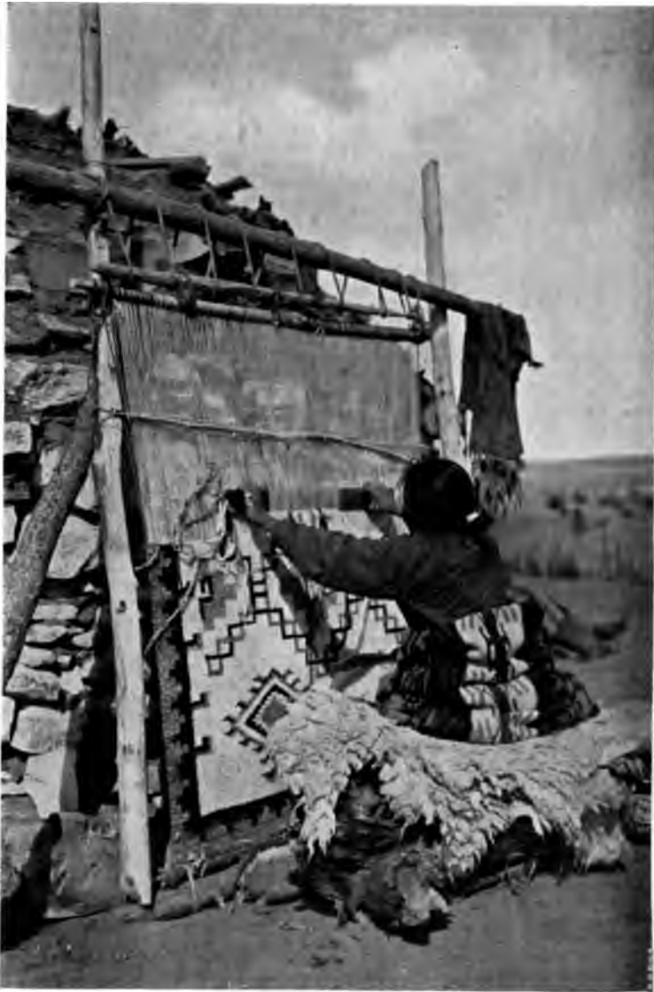
Fig. 19. A Navajo Weaver A typical New World loom. The weaving proceeds upward Goddard, 1913. I
